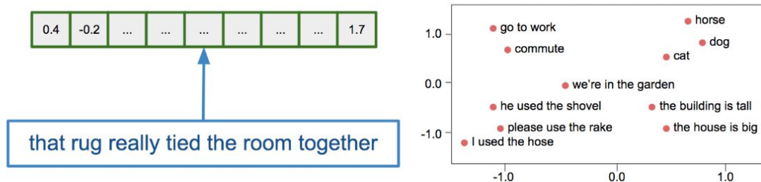
Figure 2: Text embeddings convert any text into a vector of numbers (left). Semantically similar pieces of text are mapped nearby each other in the embedding space (right).
